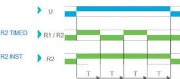
Function Di - Symmetrical flashing (ON Start)
