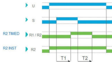
Function Ac - On/Off Delay (Delay on make/break)
