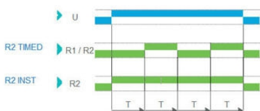
Function D - Symmetrical flashing (OFF Start)
