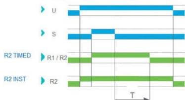
Function C - Off-Delay (Delay on break)
