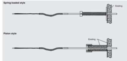
Fixed connection (compression fitting) to the furnace
