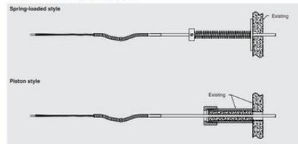
Fixed connection (compression fitting) to the furnace
