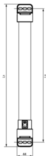
LED 021 (Size 1) L1 = 400 mm L2 = 375 mm
